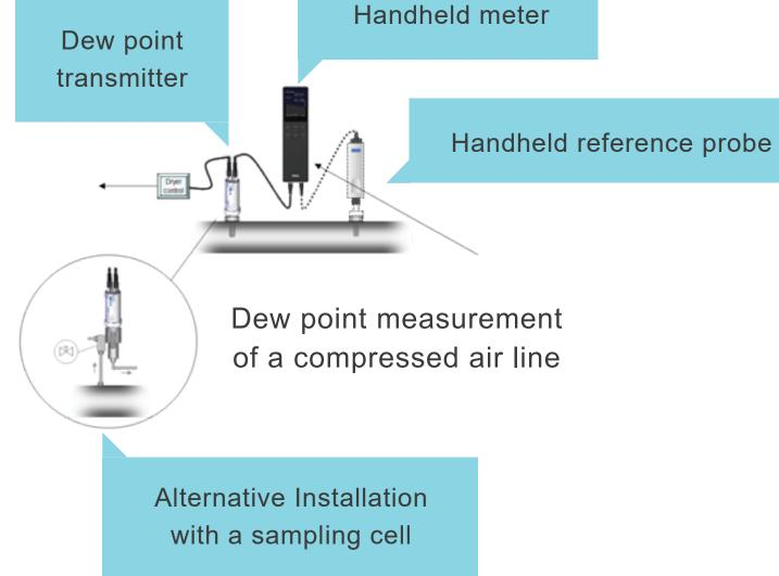
Sample cell hardware, such as quick connect fittings, a cooling coil, and welded compression fitting makes it easy to install a dew point sensor in any process.
