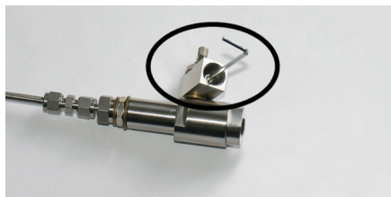
Figure 26 Removing the leak screw
