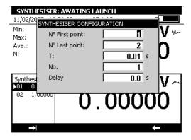
The number of the first point may be higher than that of the last point. All points between the first and last are generated.
