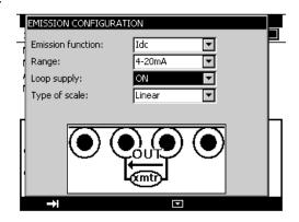
If the loop power supply is off, the MC 75.2 simulates a passive transmitter supplied with 24 V externally.
