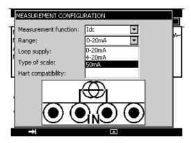
There is a quicker way to select items from a drop-down list by using the Up/Down navigation keys to select the next/previous item from the list without displaying the contents of the list. For example, the state of the "Power supply loop" field can be changed from OFF to ON using the Down and Up navigation keys.
