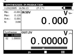
It is possible to transmit points manually one by one using the navigation keys. Use the Up and Down keys to select a point. ENTER transmits the selected point and Left / Right select and transmit the previous / next point in the list immediately.
