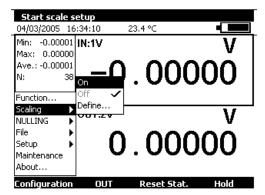
The lines entered are sorted according to increasing X to set to scale a value X, the unit searches for the 2 lines n and m=n+1 that enclose it and extrapolates linearly:
