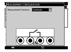
The MC 75.2 makes a resistance measurement in this mode and displays "open" if the resistance measured is greater than 1000  $\Omega$  and "closed" if the resistance measured is less than 1000  $\Omega$ .
