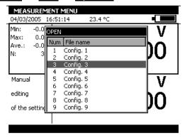
To erase the configurations of the MC 75.2, open the maintenance mode (Password 9456).
