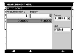
The Format and Units zones are used to select the number of decimal places and the display units.
