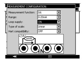
In this case, the MC 75.2 supplies a passive transmitter with 24 V and at the same time measures the current established by the transmitter.
