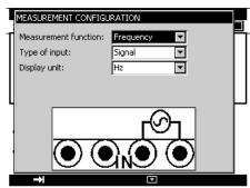
A square wave signal is generated from the input signal by comparing the amplitude of the input signal with 1 Volt. The result of the comparison is input to a microprocessor which measures the frequency by counting with respect to a very stable reference signal.
