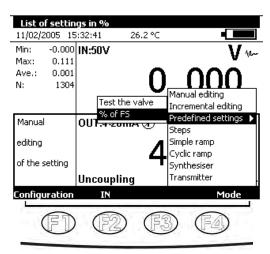
The tabulation key is used to select the next item from all the items in the dialogue box. For example, to select the "Type of scale" field on the following screen, press the key once.
