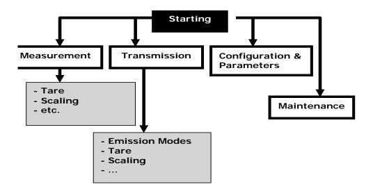
The Start procedure checks that the unit is working correctly and initialises the various tasks that are continuously executed during operation of the MC 75.2.
