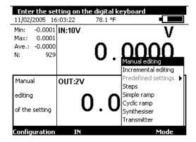
When the transmission window is open, the MC 75.2 is set by default to the Manual editing mode.
