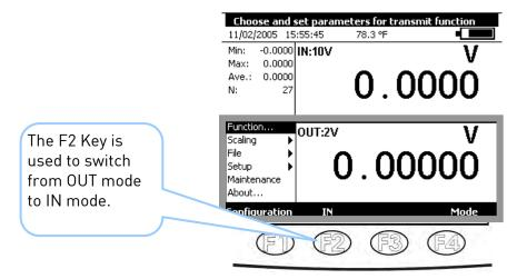
To select a Simulation function, press the **F1** (configuration) key.
