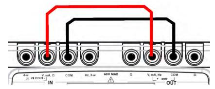
Check that the measurement displayed is the same as the simulated voltage.
