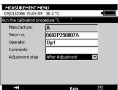
Where the procedure is executed manually, the user will have to confirm the calibration points one by one.
