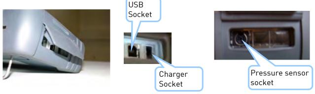
The connector for the pressure sensor is located on the right-hand side of the unit.
