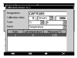
Between 1 and 4 calibration points can be entered per sensor.
